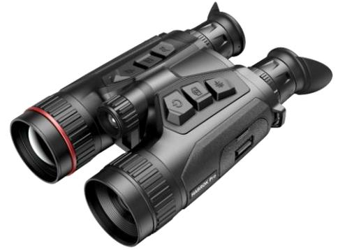
HIKMICRO HABROK Pro HQ50LN multi-spectrum binocular is equipped with an 15 mK NETD, 640 × 512 thermal detector @50 mm thermal lens and an advanced 4K digital detector with 60mm lens, ensuring perfect image quality and detail recognition in various weather and light conditions. Combined with a 1000 m Laser rangefinder and replaceable IR emitter @940 nm wavelength, this all-in-one binocular can be applied mainly in forest & field hunting, birding, animal searching, rescuing and marine scenario.
