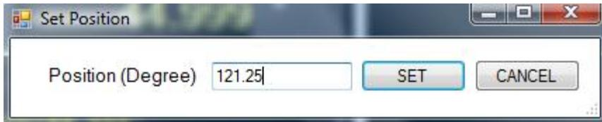
Input the known position angle into the box in degrees and press SET. You will notice that the location on the display window does not change but the value will change. Also notice that the number scale on the top has moved to represent the new position angle.
