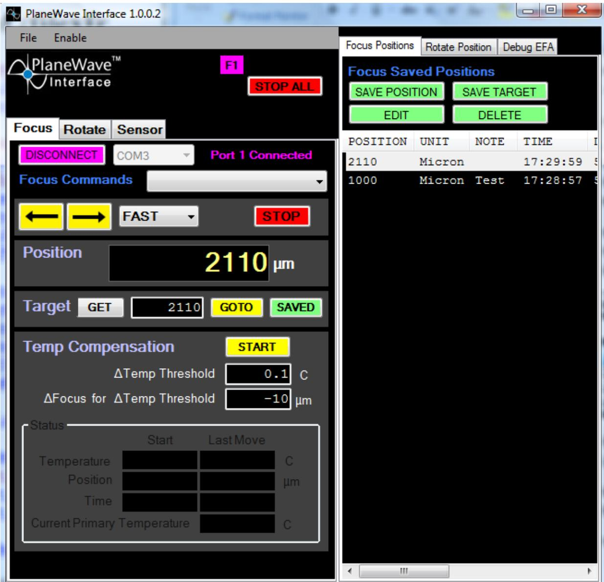
**8 – GOTO:** When this button is pressed, the focuser or rotator will move to the position in the Target window.
