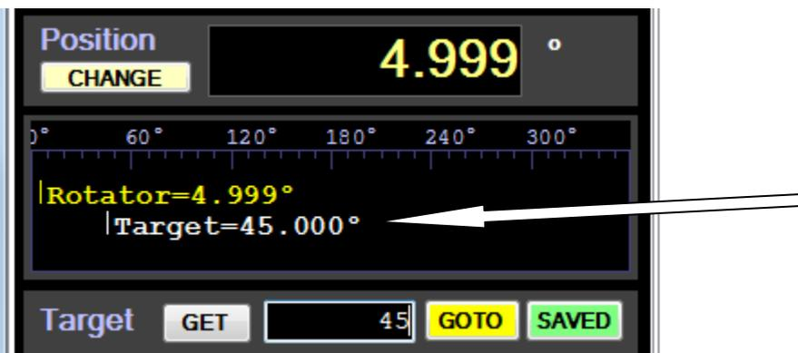
If you press the GOTO button, then the GOTO position will also appear in the Position Window until the rotator reaches the target, see below.
