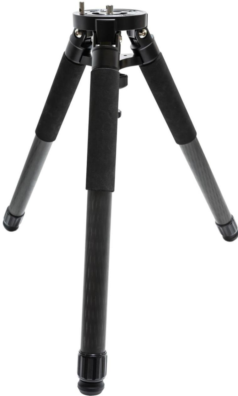
iOptron Carbon Fiber tripod (#8061) has 10 M6 threaded holes and a M12 hole in the middle for center post. The tripod rod has a 3/8"-16 thread.
