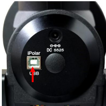
Figure 25. Connect CEM70 iPolar to a computer
