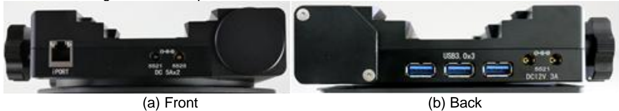
Figure 4. Ports on CEM70G dovetail saddle
