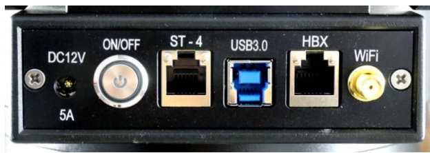
Figure 2. Ports on a CEM70G mount base
