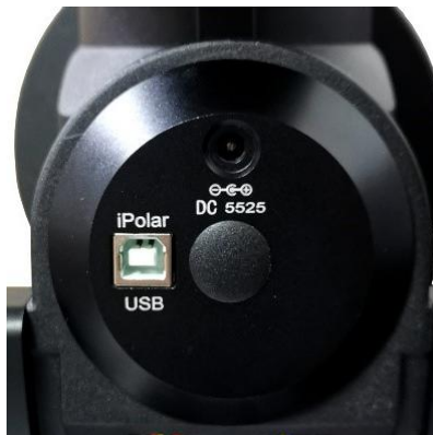
Figure 8. iPolar/USB and DC input on the rear end of RA axle
