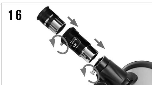
To use the Barlow lens, remove your eyepiece from the telescope focuser, insert the Barlow lens into the focuser and insert your eyepiece into the Barlow lens. This will double the magnification of whatever eyepiece you use it with.
