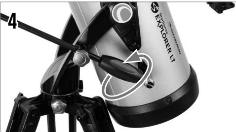
Fine adjustment in the up-and-down direction can be done using the altitude slow motion rod. Keep the rod guide knob locked and rotate the black handle on the slow motion rod. This allows you to move the telescope in small increments to help center objects or follow celestial objects in the night sky.
