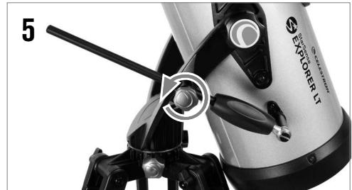
The altitude slow motion rod has a limited range of motion of about 15 degrees. If you run into the end of travel and the knob will no longer turn, you can reset it by loosening the rod guide knob and turning the slow motion rod handle the opposite direction until you are in the middle of its travel, then retighten the rod guide knob.
