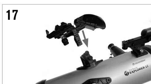
To install the StarSense smartphone dock, loosen the two setscrews on the dock mount on the top of the telescope tube and slide the dovetail on the bottom of the dock into the mount. Secure in place by tightening both screws.
