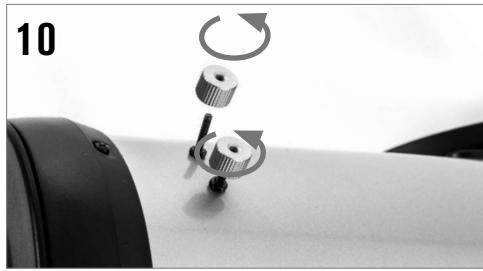
To install the finderscope, remove the two silver nuts from the threaded posts on the top of the tube, near the focuser.
