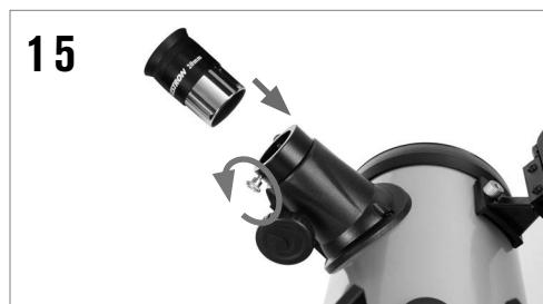
To install the eyepiece, loosen the setscrews on the focuser. Insert the silver barrel on the bottom of the eyepiece into the focuser and secure by tightening the setscrews. Always start using your low-power eyepiece (25 mm) to help you find the target you wish to view. You can always change to your high-power eyepiece (10 mm) later.
