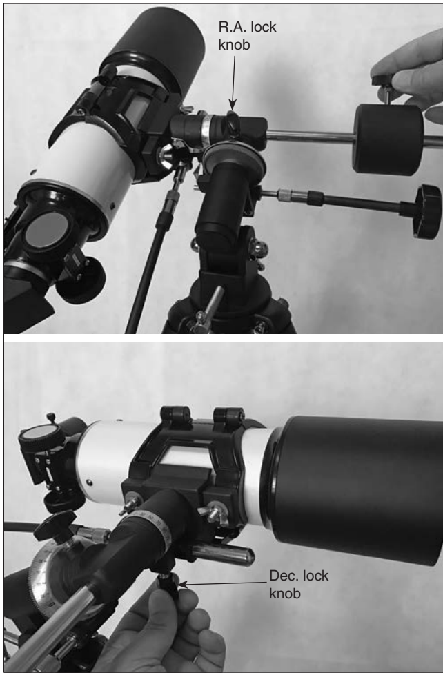
Figure 14. To balance the telescope on the mount, you first A) balance it on the R.A. axis, then B) on the Declination axis.
