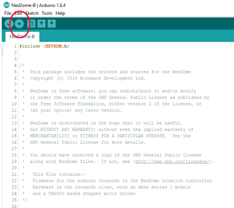
Figure 11: Firmware upload to Arduino. Simply press the upload button after opening the file with the software.
