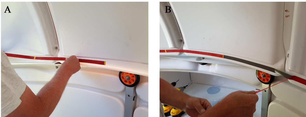
Figure 1 Install the double-sided tape as in (A) and remove the protective cover strip (B).
