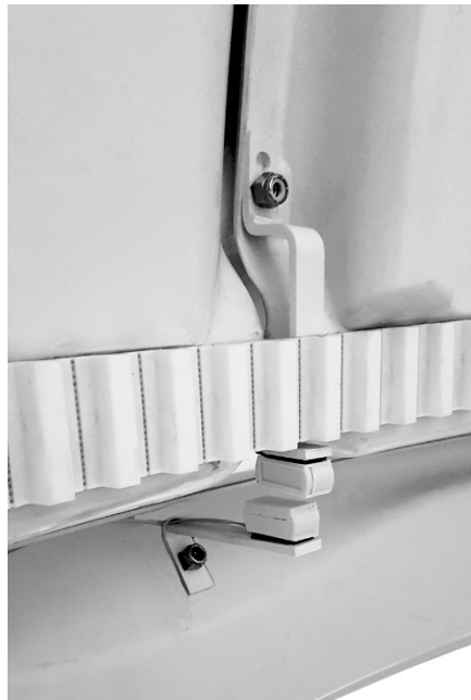
Figure 4: placement of the magnetic switch and magnet.
