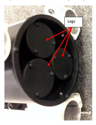
4. Install the leg onto the Tri-pier leg house. Make sure the feet locking screw is aligned to the Leg Adjustment & Leveling Screw.
