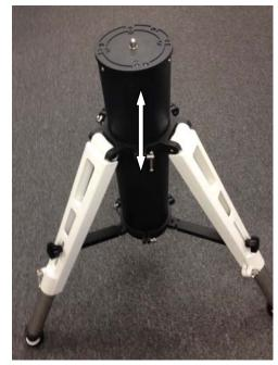
8. Adjust the Tri-pier legs by spreading the legs. Make sure that the Tri-pier feet are sit inside the vibration suspension pads. The pads and the ground surface are contacted well. Tighten the Leg Adjustment & Leveling Screws to secure the Tri-pier.
