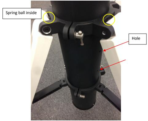
7. Move the Center Column up or down to desired height until hear the "click" sound. Lock the Pier Height Adjustment Levers.
