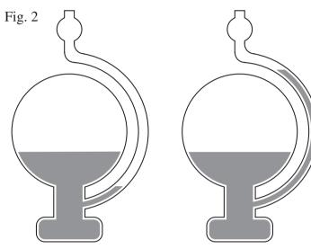
Low water in the spout indicates high air pressure, expect fair weather High water in the spout indicates low air pressure, expect stormy weather
