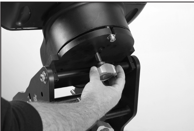
Figure K. Attaching the center mounting bolt.
