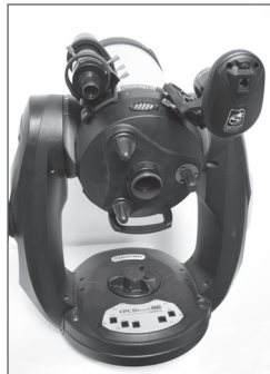
Finder and StarSense installed on CPC 800
